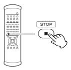
Press the STOP button (the ring surrounding the STOP button on the main unit lights).
